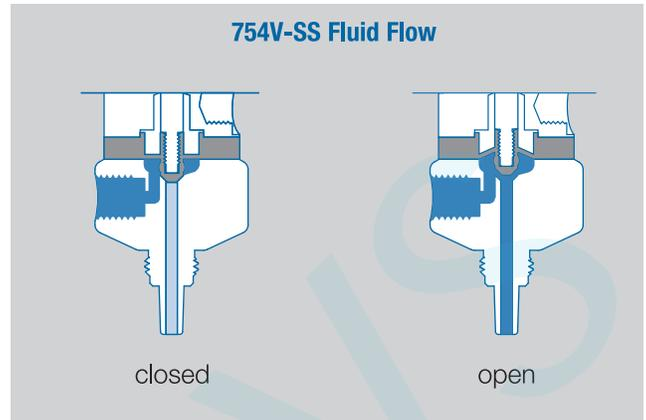
The primary control of deposit size is the valve open time.
