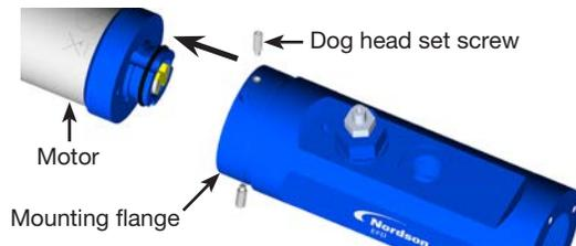
2. Unscrew and remove the mounting flange.
