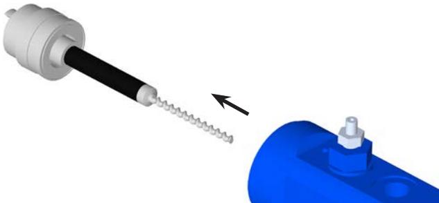
4. Carefully isolate the seal bearing assembly from the rotor.
