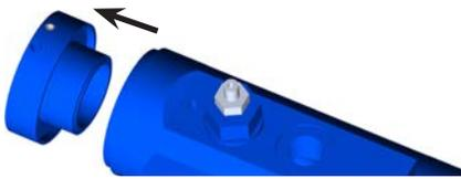
3. Remove the seal bearing and rotor assemblies.
