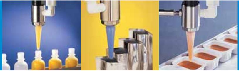
The complete system includes the 725HF dispense valve, ValveMate™ 8000 controller, the fluid reservoir and dispense nozzle.
