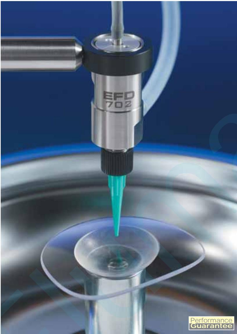
The 702V-SS mini-diaphragm dispense valve is designed for drip-free coatings and consistent shot-to-shot bonding of UV-cure adhesives and other low-to-medium viscosity fluids, especially where valve mounting space is at a premium.
