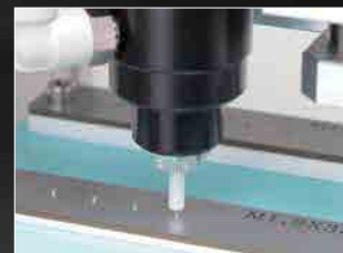
Tightens screws as small as M1.0.
