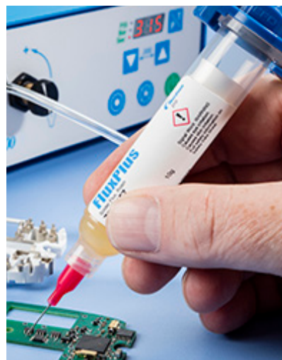
Performus™ X100 dispensing FluxPlus onto a PCB.
