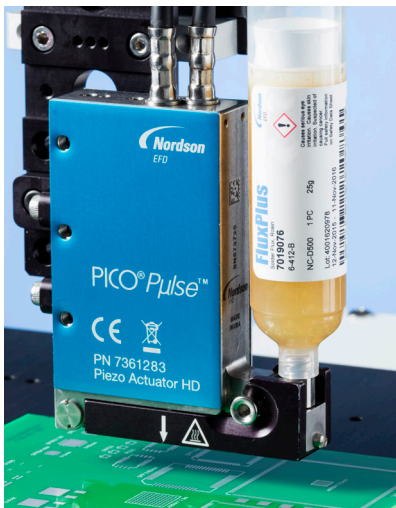
PICO Pulse® jetting FluxPlus onto a PCB.
