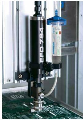
794 auger valve dispensing accurate, repeatable amounts of EFD solder paste onto printed circuit board.
